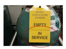
Indicates an IN SERVICE compressed gas cylinder
