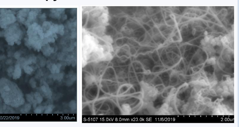
The average particle size of alumina nanopowder of (150± 20) nm (left) while the diameter of CNTs is  $(35 \pm 15)$  nm (right).
