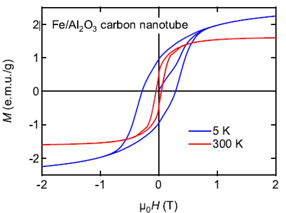
The Fe- catalyzed CNT/Alumina nanocomposites show a strongly pronounced hysteresis curve as compared to diamagnetic response from  $Al_2O_3$ .
